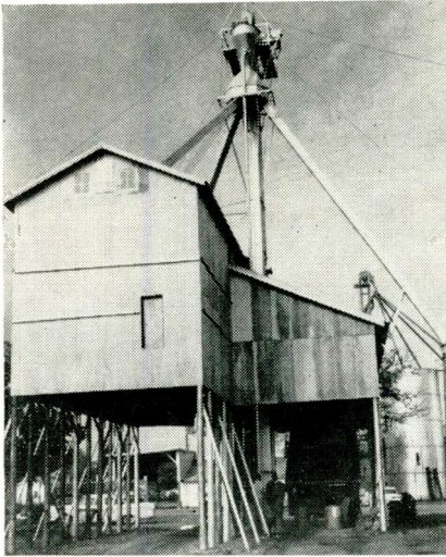
Fig. 19: Spout-type automatic sampler draws samples of peanuts as they flow by gravity through the discharge spout of a belt and bucket elevator.
