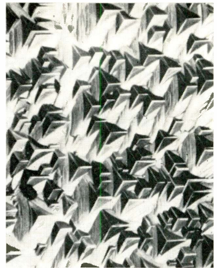
Typical epitaxial growths, ranging in thickness from 25 to 800 microns, deposited on the (111) surfaces of silicon substrates are shown at a magnification of 400.
