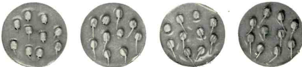
Fig. 9: Corn germinated faster after exposure at less than atmospheric pressure to low frequency radiation. Seeds at left were not treated; the others were treated at 4, 8, and 16 ma, respectively.
