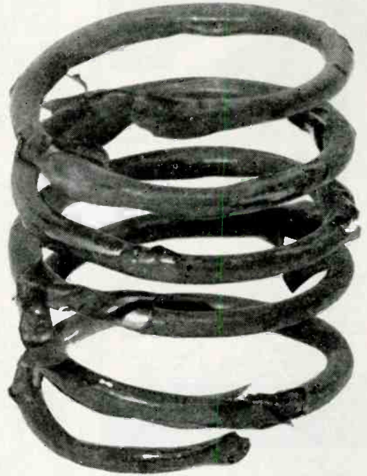
This "Glyptal"-insulated wire was exposed to ordinary chlorinated solvent for the same length of time as the one on the left. The solvent dissolved the resin binder and softened the alkyd finish.
