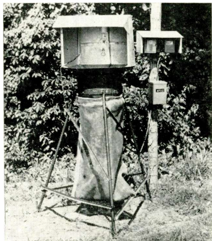
Fig. 17: Insect traps such as this can be powered by a transistorized power supply, thus extending their use to areas where line extension cost might be prohibitive.
